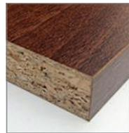
The vast majority of office furniture is manufactured with this material. MFC is usually of a wood grain, which is repeatedly printed onto a Melamine film, and heat processed onto chipboard. MFC is a budget alternative to High Pressure Laminate table tops only suitable for I.T. benching.
