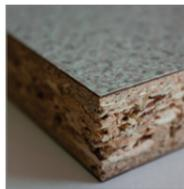
Typically used on kitchen worktops and classroom tables, in different grades. Usually referred to as a laminate top and bonded to either MDF board or chipboard. The layer of laminate is adhered to the substrate (the board) under high pressure. It is very resilient to knocks and abrasions, is very hygienic.
