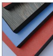
SGL (also referred to as Compact Grade Laminate or as "Trespa" which is a trade name) has a solid core built up from multiple layers of resin-impregnated high quality kraft papers to thicknesses between 2mm and 20mm. It is suitable for use in both wet and dry areas making it a great choice for science and washrooms.
