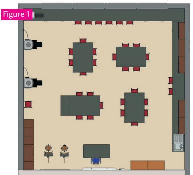
The illustrated layout is fully compliant with Building Bulletin 81.
