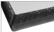
A relatively new process, spray PU is sprayed onto an MDF top. It is 2mm thick, and a flexible process and therefore can be applied to more shapes than cast PU however, making it a favourite with manufacturers.
